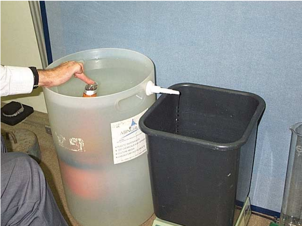
Photo 5. The set-up for testing procedure 3 – Beacon submerged.
