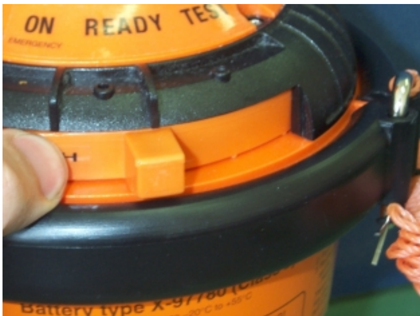
Photograph 4, shows thumb applying pressure to lever slide.
