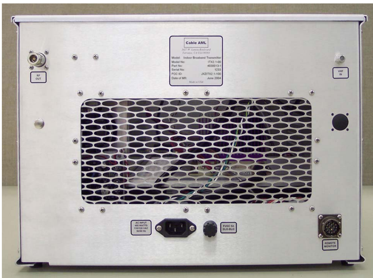
Figure 8. Outside ID Label Location.
