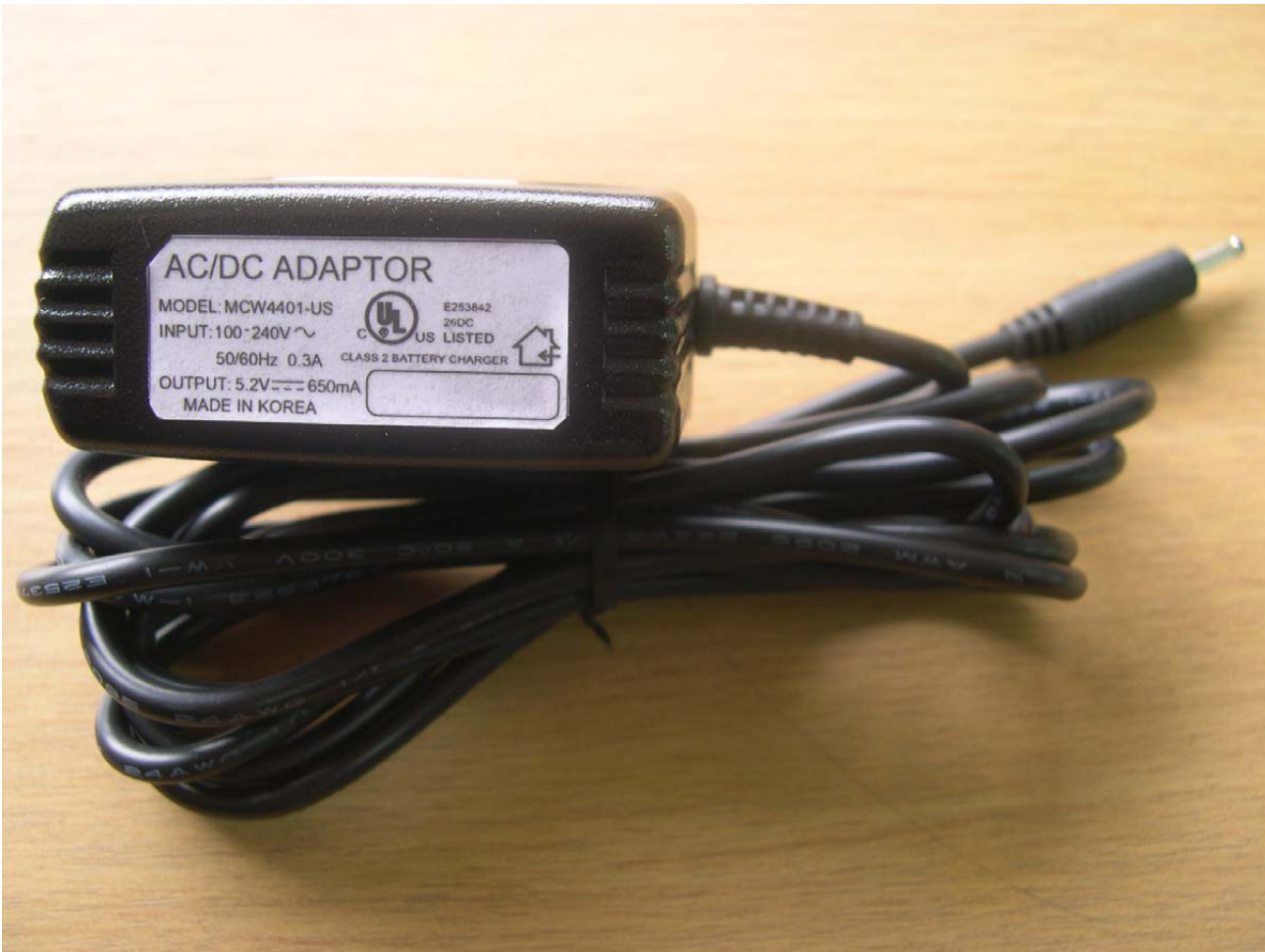
<Photograph 5: AC/DC Adaptor #3> Model MCW4401-US Manufacturer: Macroway Technologies, Inc.
