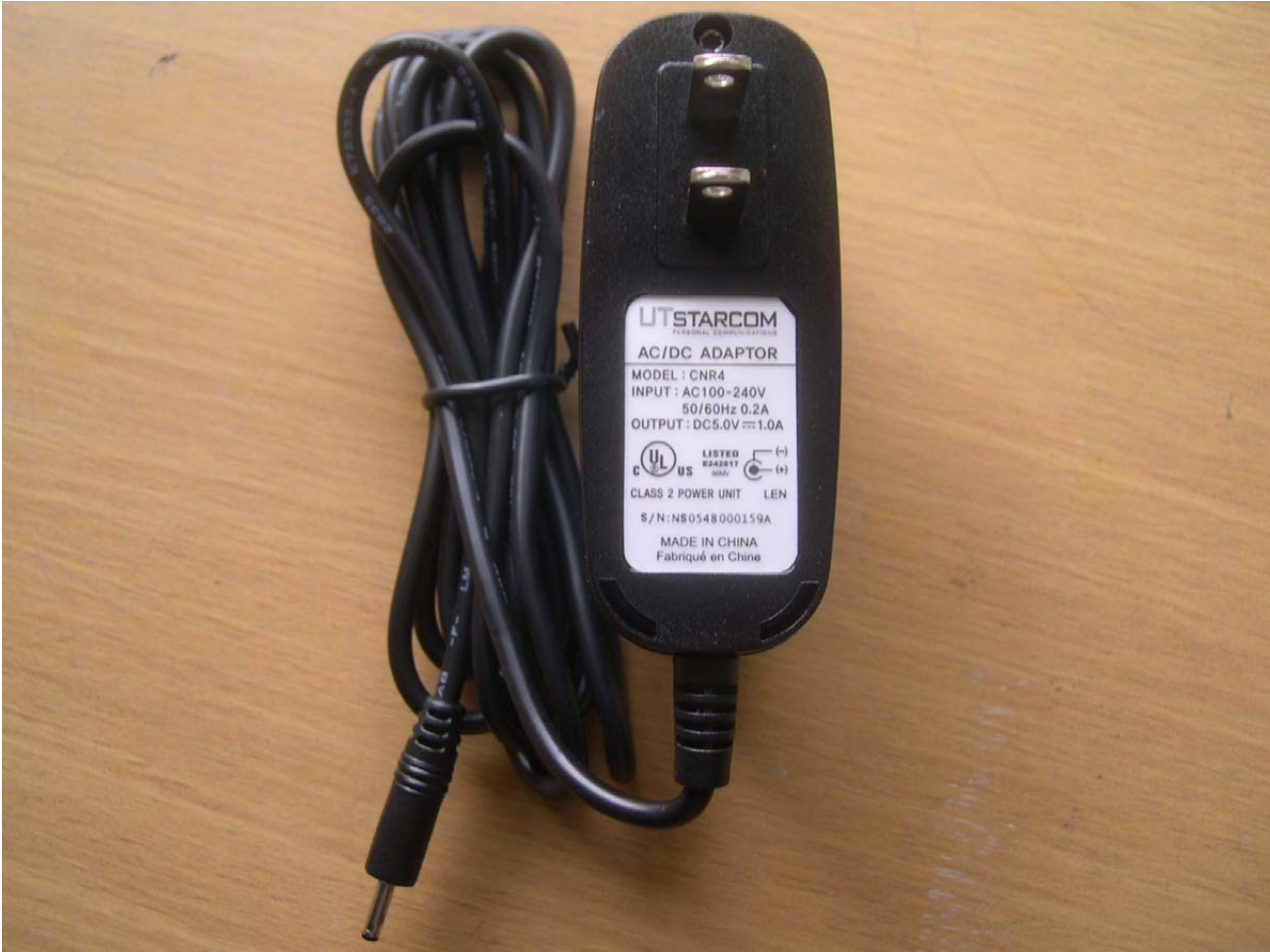
<Photograph 7: AC/DC Adaptor #5> Model CNR4 Manufacturer: Chang Shung International Co Ltd
