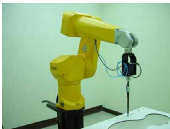
Fig. 5.2 Probe setup on robot
