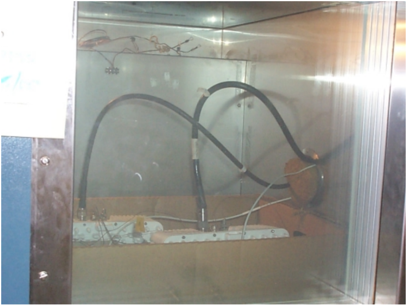
Figure 54: Frequency stability testing EUTs (SUB and HUB) in the Temperature chamber.
