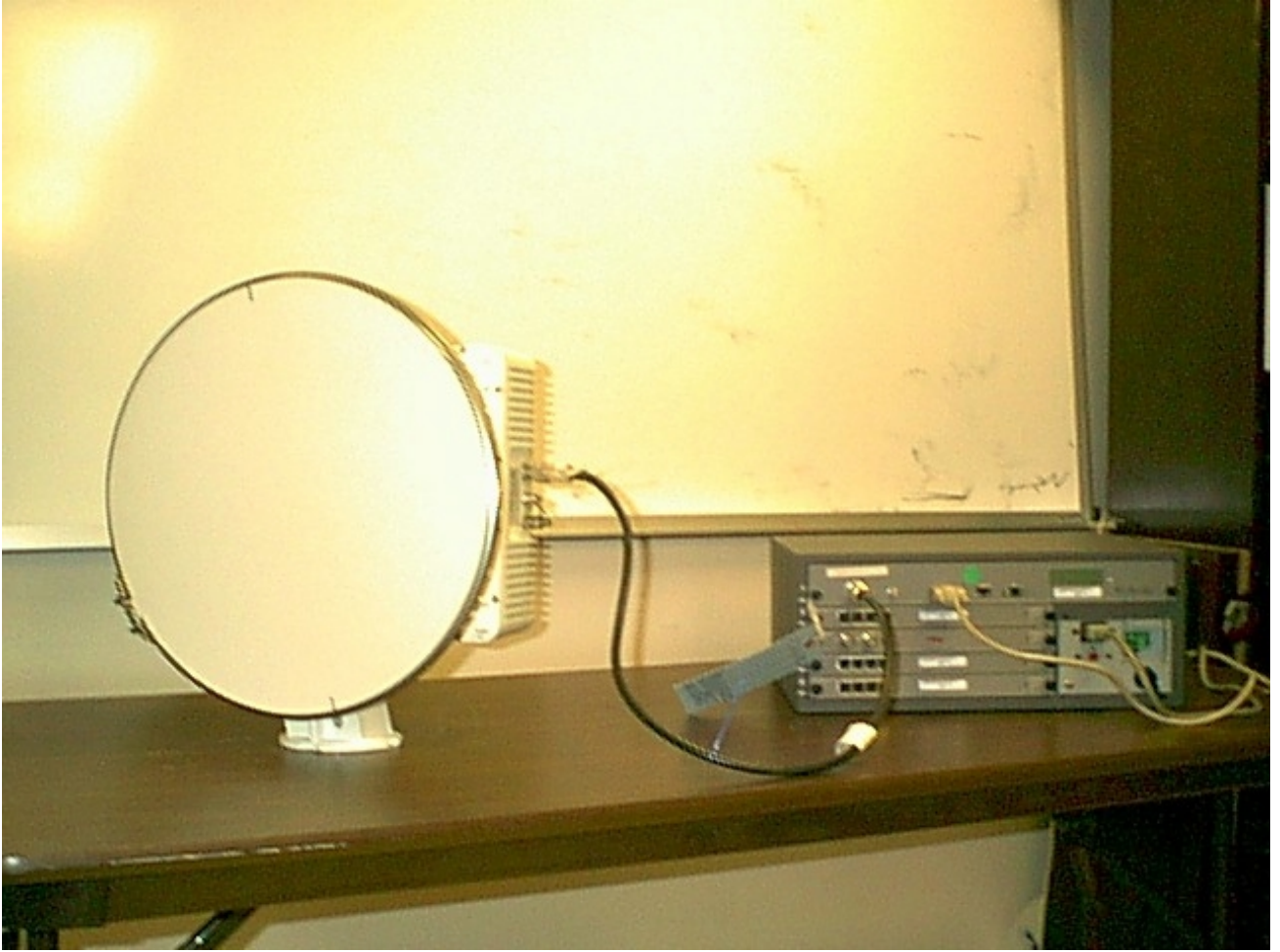
Figure 3 ODU and IDU – Front View
