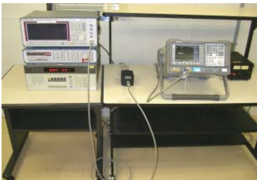
Unwanted Emission Replace Method (Conducted Spurious)
