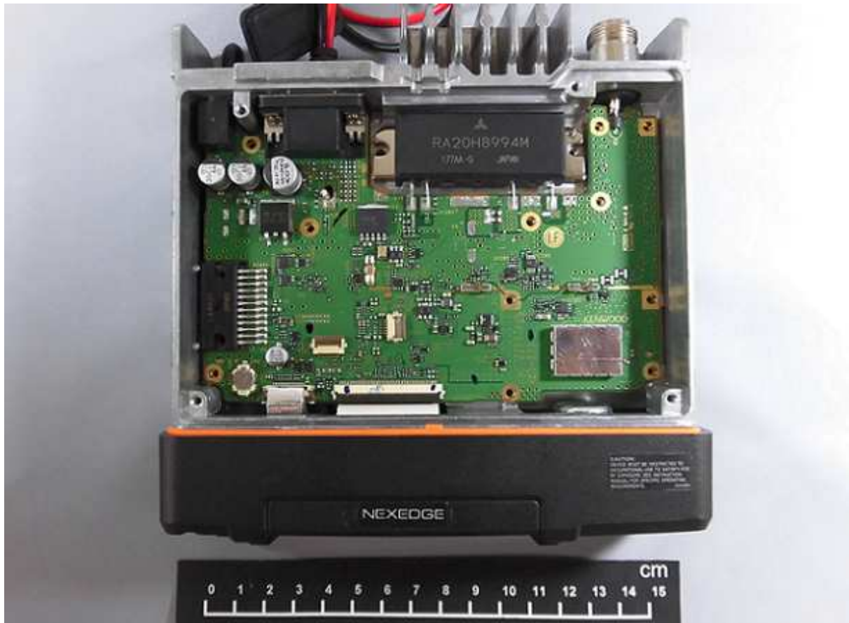
Top Internal View of TX-RX Unit
