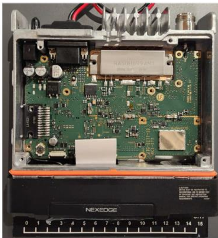
Top Internal View of TX-RX Unit
