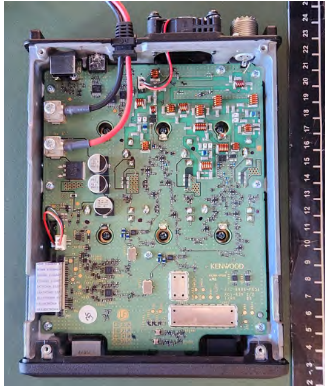
Top Internal View of TX/RX Unit
