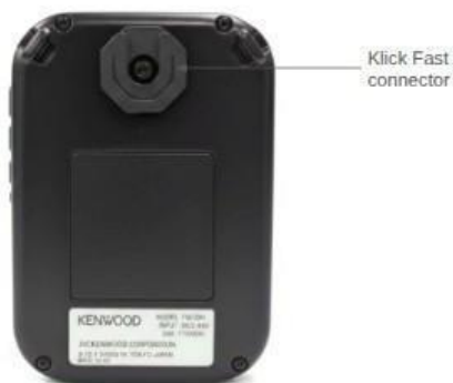
Figure 24. Click Fast connector behind the device
