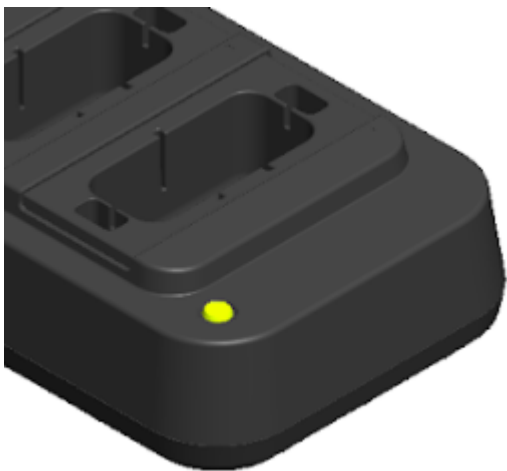
Figure 23. DOCK Yellow LED for moisture or temperature fault
