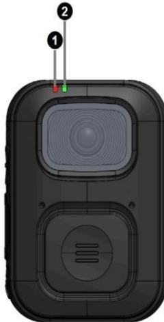
Figure 17. Front View of the Device Showing Both LEDs
