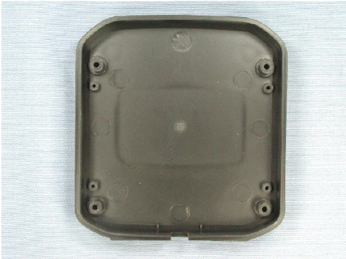
Inside Bottom of Battery Charger without PWB
