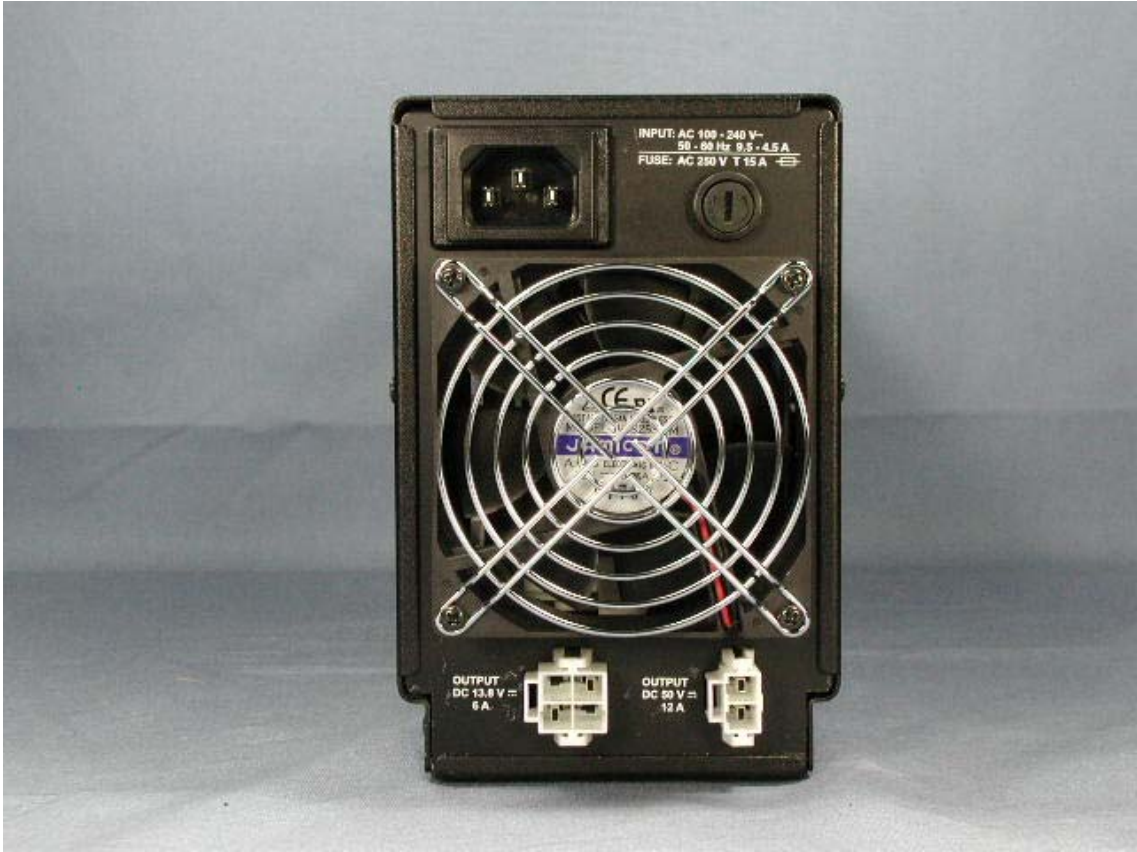
Rear view of power supply
