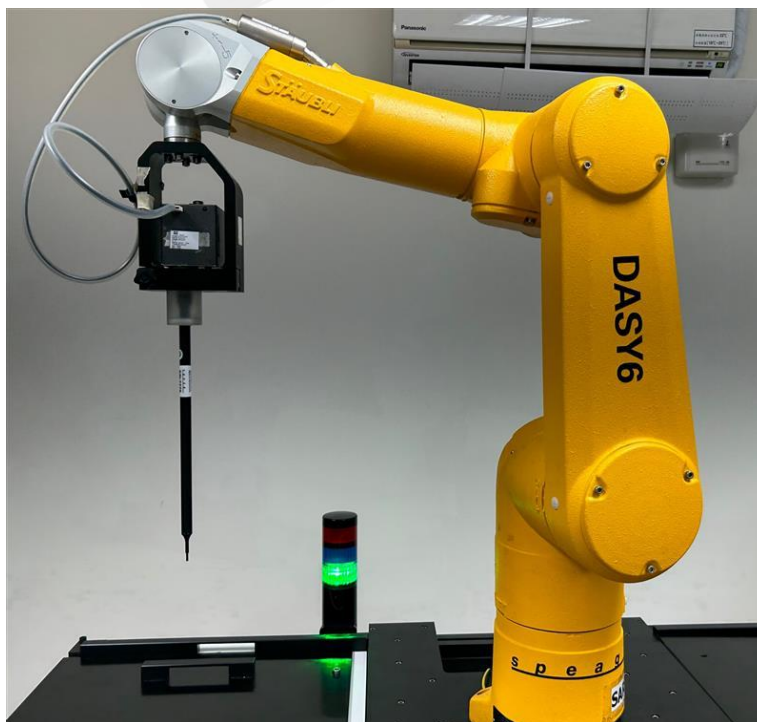
Fig.1 Photograph of the SAR measurement system
