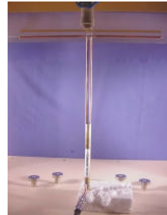
300MHz System Check Setup Photograph
