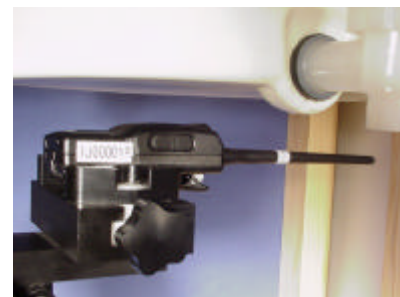
Face-held SAR Test Setup 2.5cm Separation Distance
