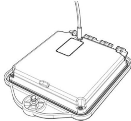
Figure 4.13 Charging the transmitter Li-Ion battery pack
