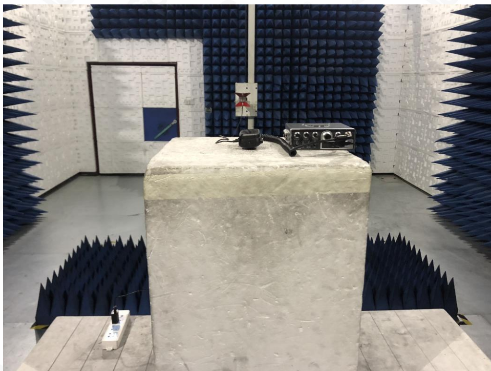
RADIATED EMISSION TEST SETUP ABOVE 1GHZ
