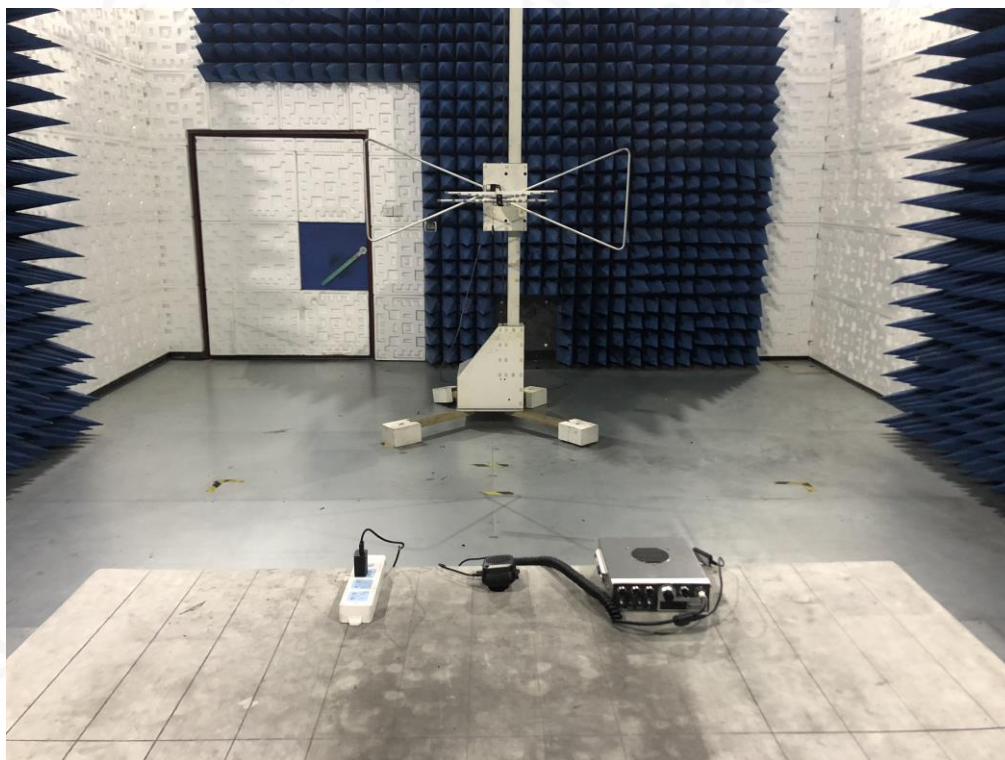
RADIATED EMISSION TEST SETUP ABOVE 1GHZ
