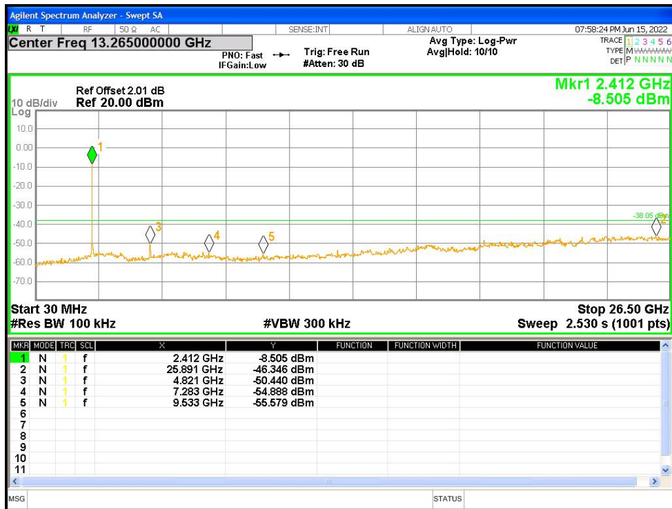
Tx. Spurious NVNT n20 2437MHz Ant1 Ref
