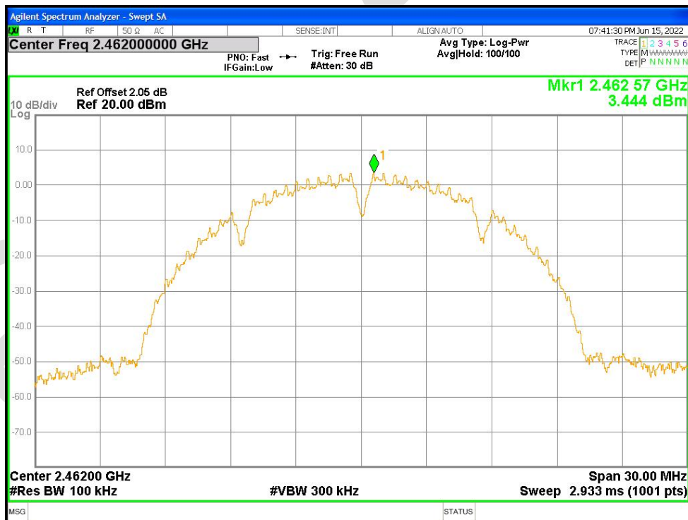
Tx. Spurious NVNT b 2462MHz Ant1 Emission
