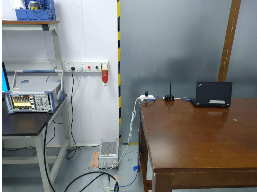
Conducted Emissions at AC Power Line (150kHz-30MHz)
