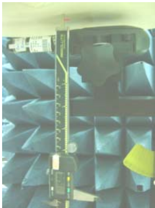
Figure 11.5 Body SAR Test Setup -----w / out Belt Clip-----
