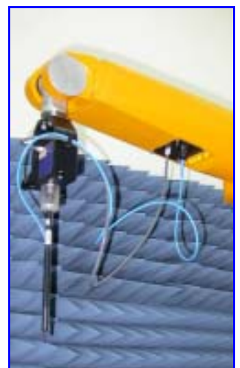
Figure 6. Probe setup on robot
