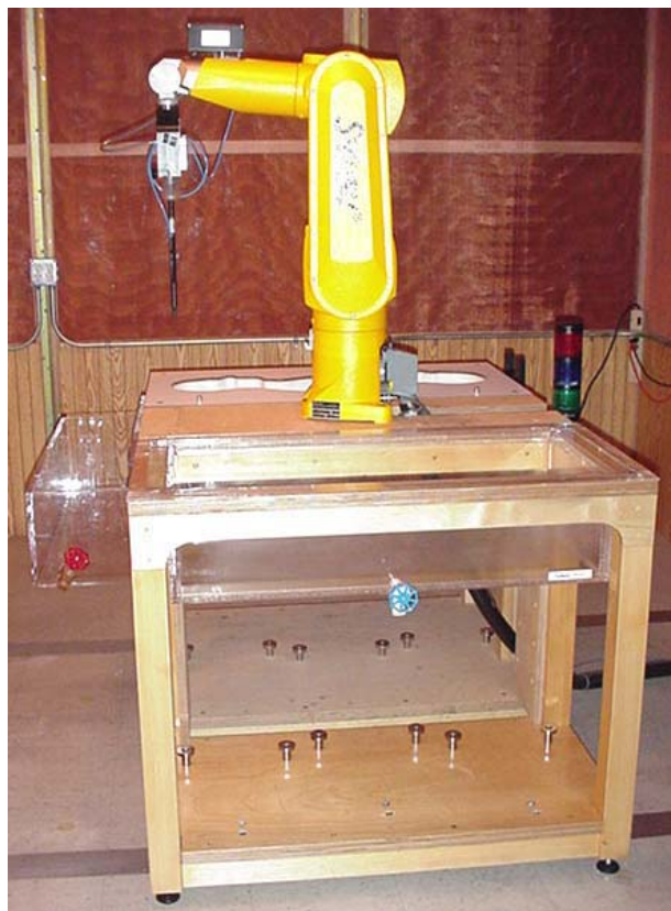
DASY4 SAR Measurement System with validation phantom
