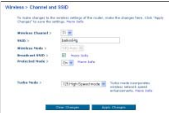
Figure 4-13 Channel and SSID
