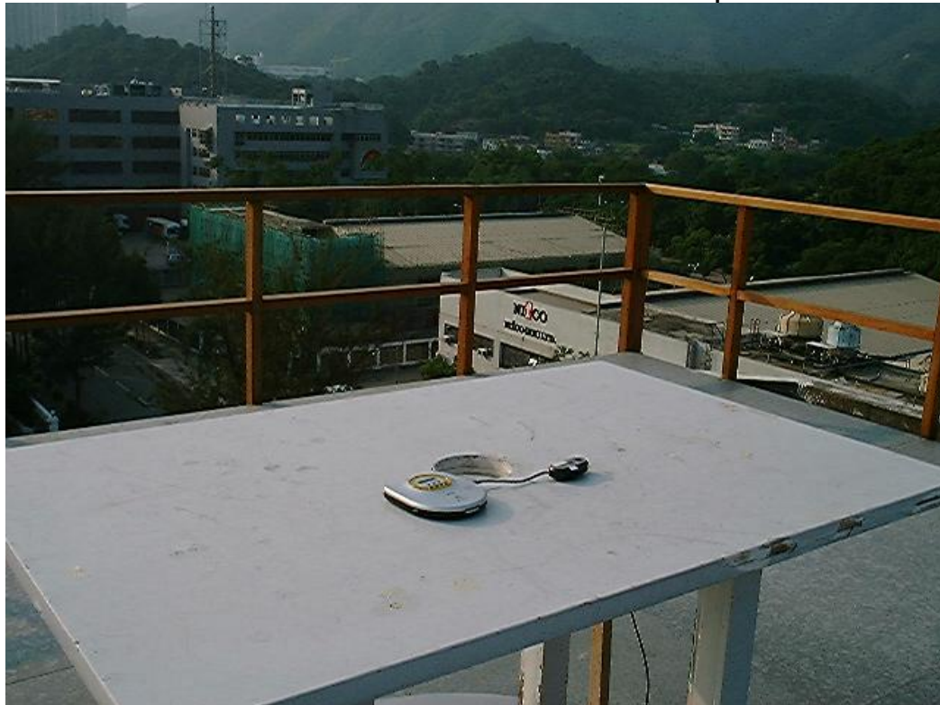
Measurement of Radiated Emission Test Set Up
