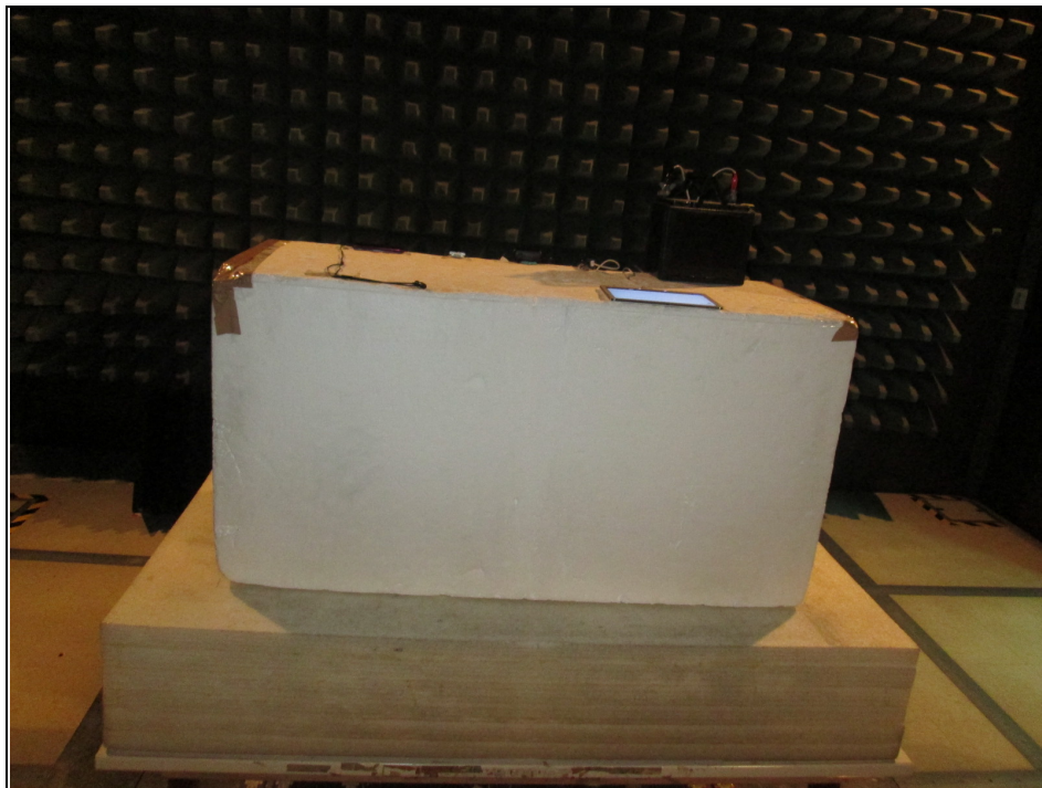
Radiated Emission Test (Above 1GHz)
