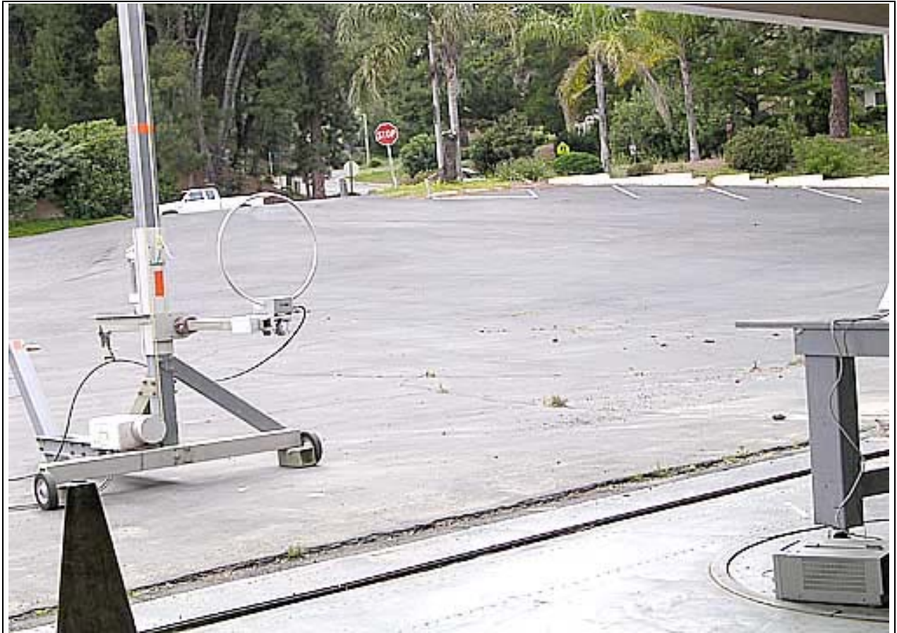
Radiated Emissions - Front View - Loop Antenna
