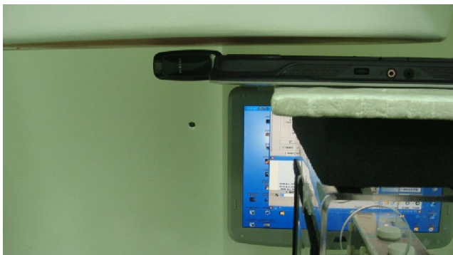
Direct Laptop Plug-in USB Configuration 4 (Vertical Back with Phantom 5 mm Gap)
