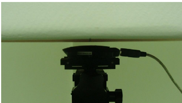
USB Cable Plug-in for USB Configuration 2 (Horizontal Down with Phantom 5 mm Gap))
