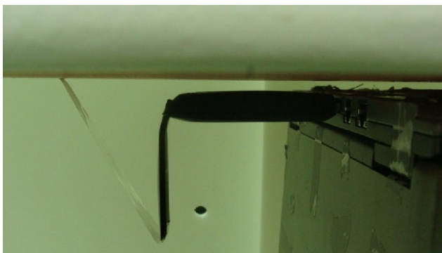
Direct Laptop Plug-in for USB Configuration 1 (Horizontal Up with Phantom 5 mm Gap and Antenna Status 90°)
