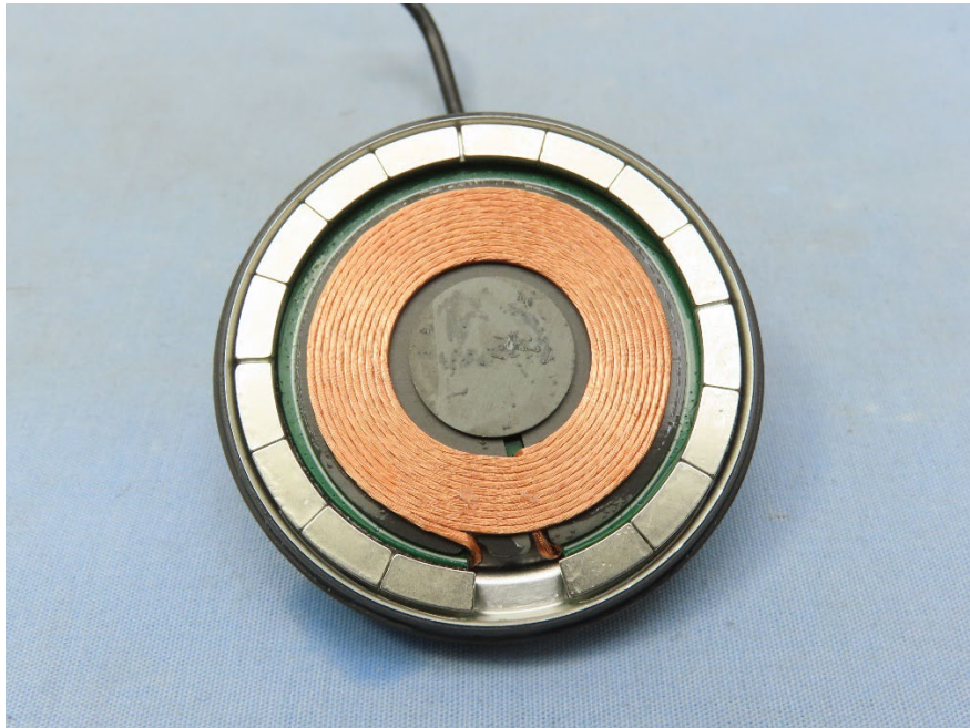
MPP Qi2 Coil (127.7kHz / 360kHz)
