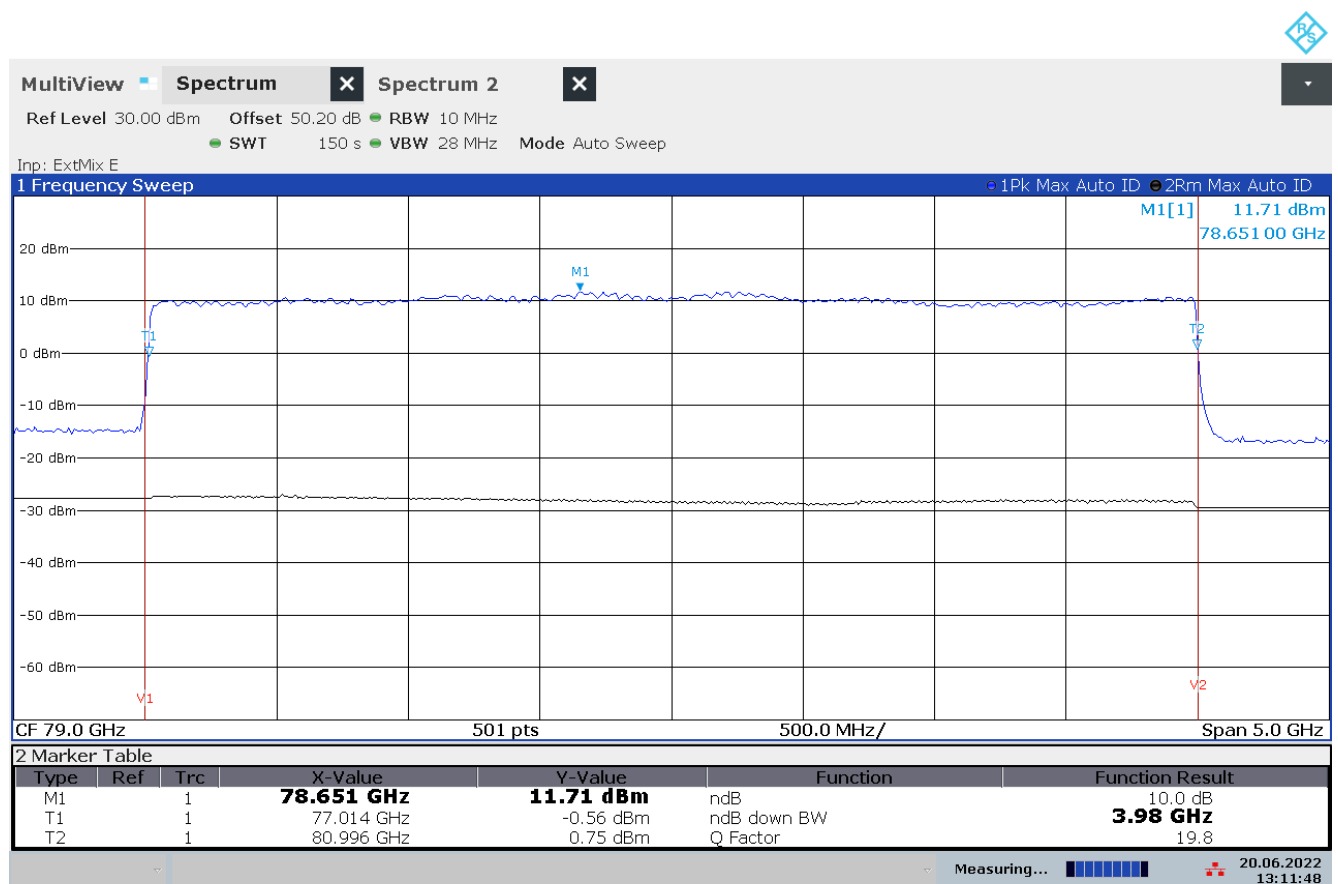
Plot 1: 10 dB bandwidth, Pos-Peak measurement, reference at 20°
