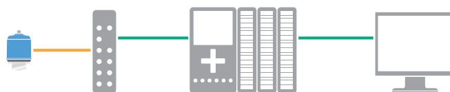
Figure 5-3: Connection via the PLC
