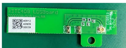
Figure 7: LDS board - top side
