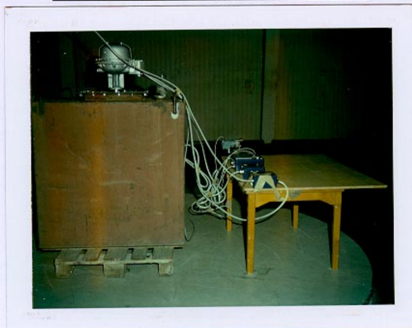
Test set-up, Radiated Emission 30 - 1000 MHz
