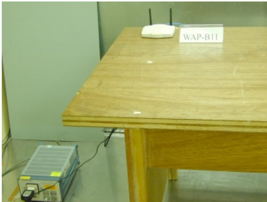
Photo 1: Conducted Test Set-up photo
