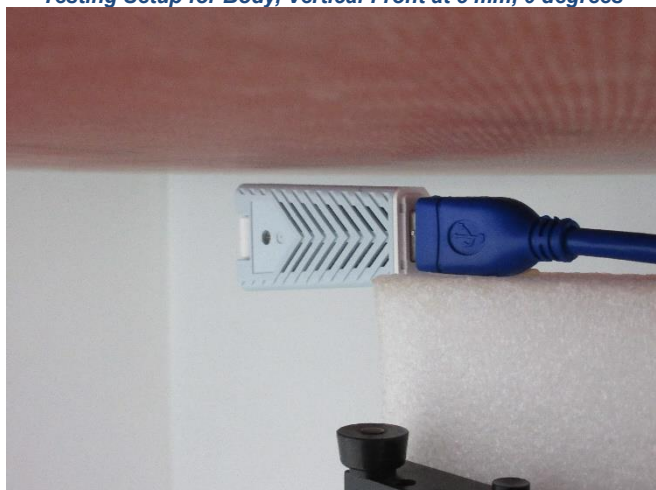
Testing Setup for Body, Vertical-Front at 5 mm, 0 degrees
