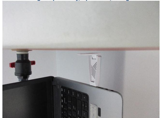
Testing Setup for Body, Tip at 5 mm, 90 degrees
