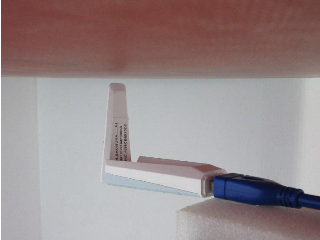
Testing Setup for Body, Horizontal-Down at 5 mm, 90 degrees
