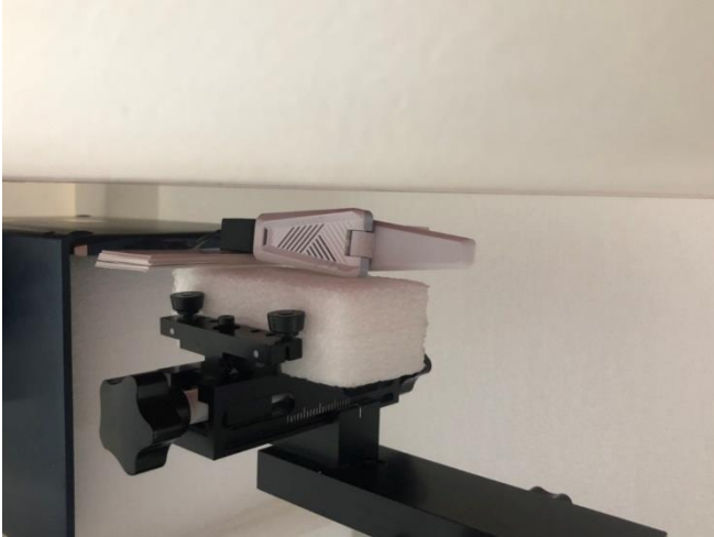
Testing Setup for Body, Vertical-Front at 5 mm, 180 degrees
