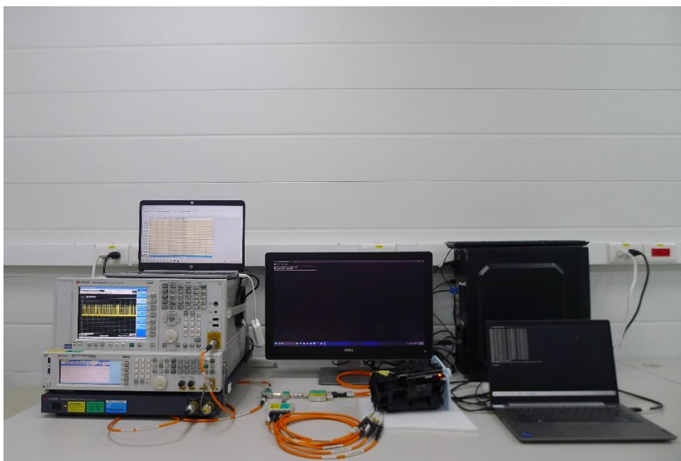
Description: DFS Test Setup_Master
