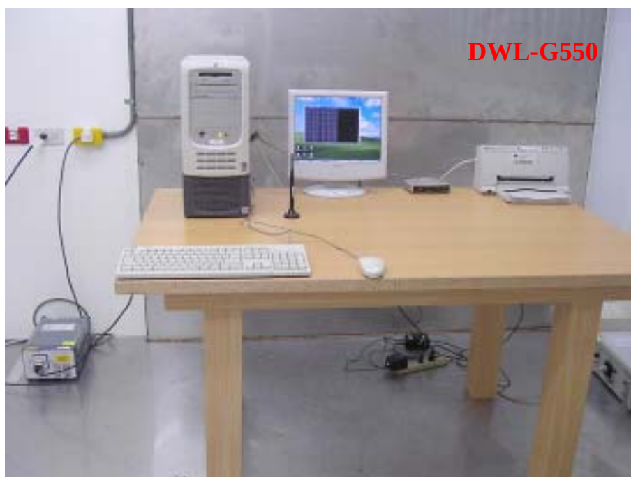
Photo 2: Conducted Emission Test Set-up
