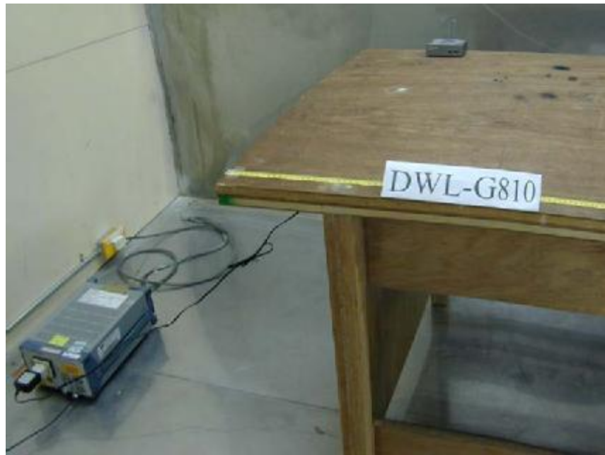
Photo 2: Conducted Emission Test Set-up
