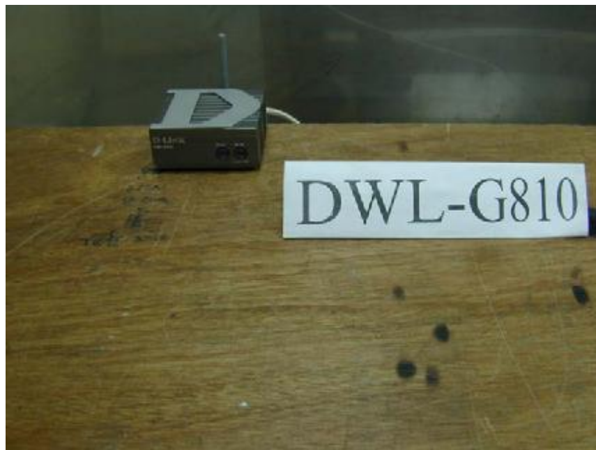
Photo 2: Conducted Emission Test Set-up
