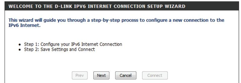
The router will try to detect whether its possible to obtain the IPv6 Internet connection type automatically. If this succeeds then the user will be guided through the input of the appropriate parameters for the connection type found.
