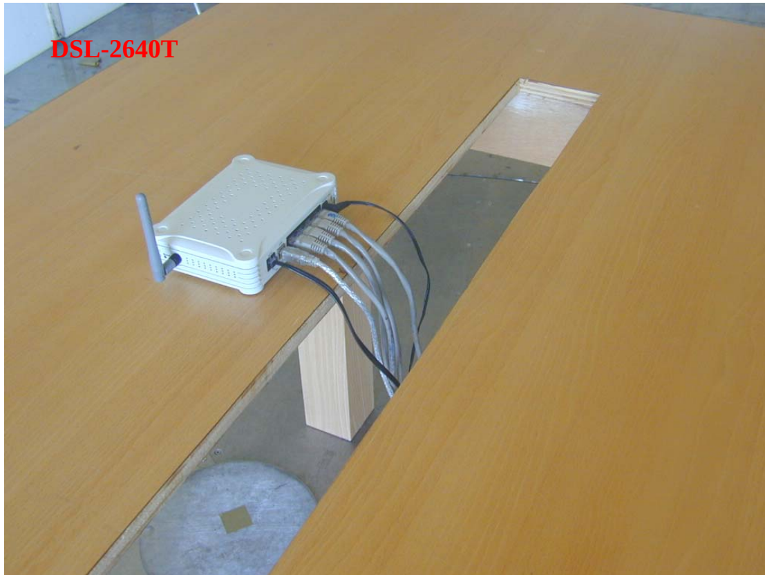
Photo 4: Radiated Emission Test Set-up
