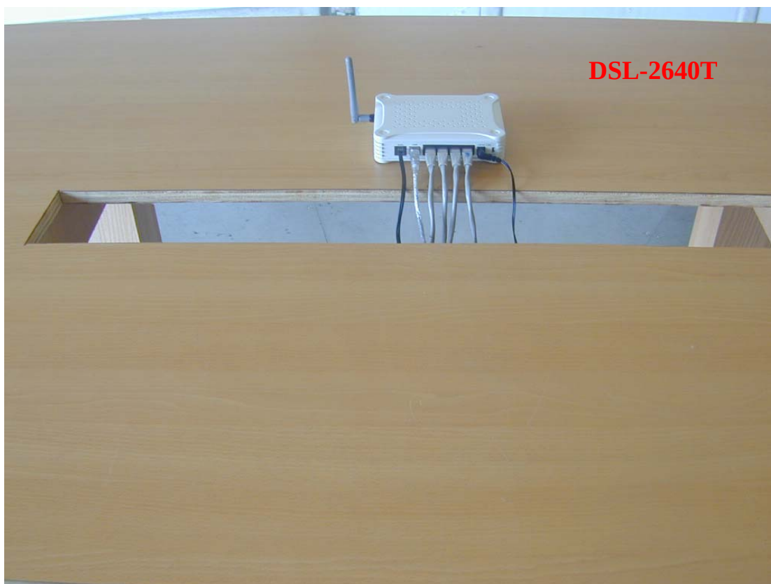
Photo 1: Radiated Emission Test Set-up
