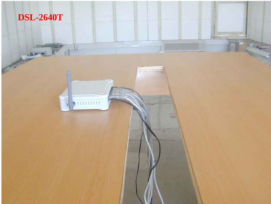
Photo 3: Radiated Emission Test Set-up
