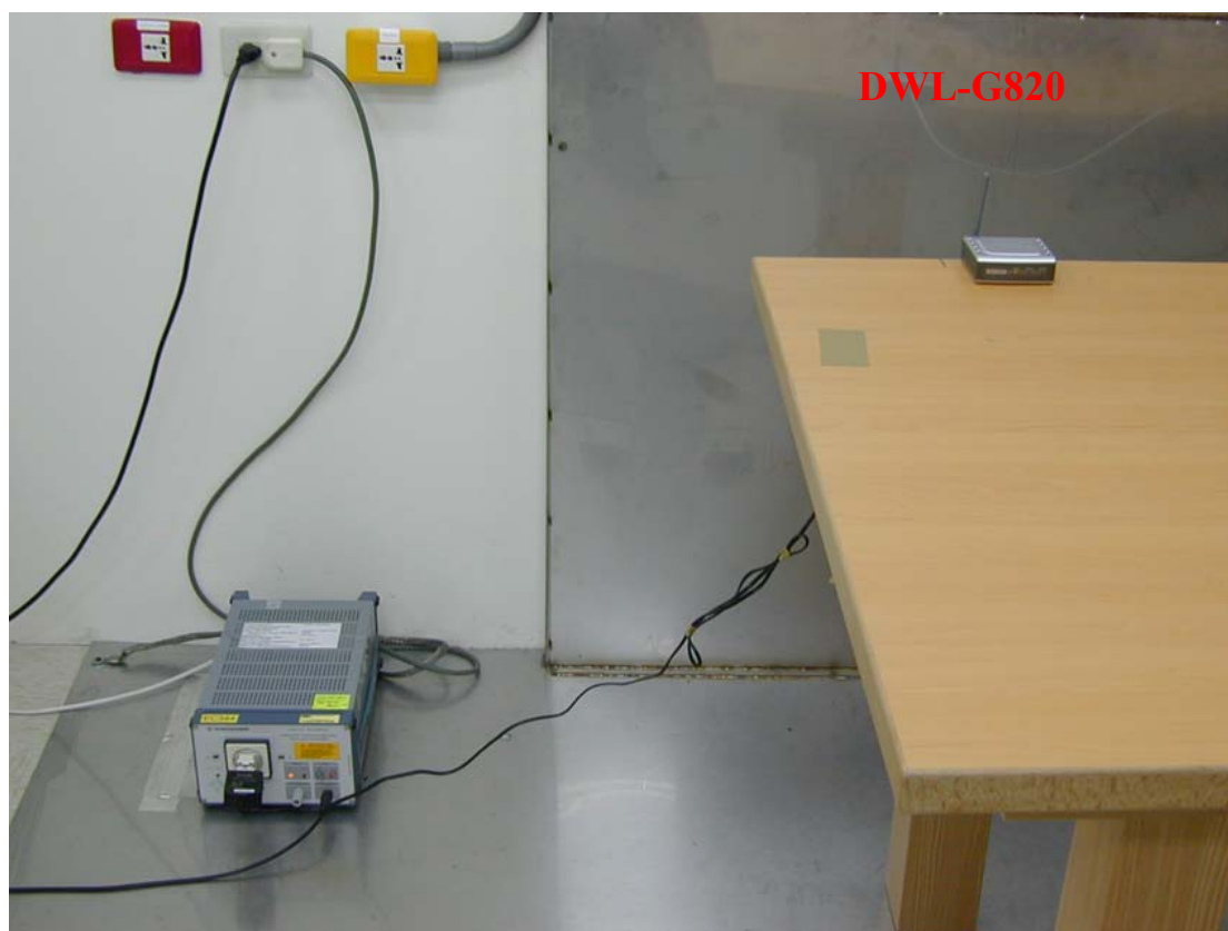
Photo 1: Conducted Emission Test Set-up
