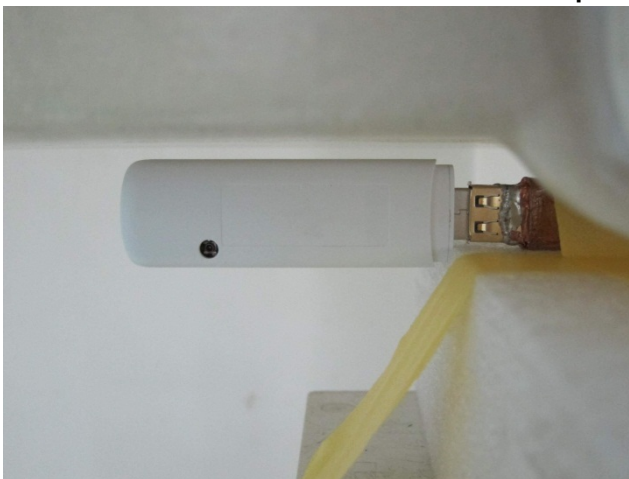
USB Cable Plug-in USB Configuration 4 Vertical Back with Phantom 0.5 cm Gap
