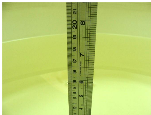
Fig 6.2 Photo of Liquid Height for Body SAR
