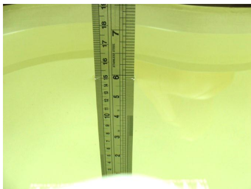
Fig 6.1 Photo of Liquid Height for Head SAR
