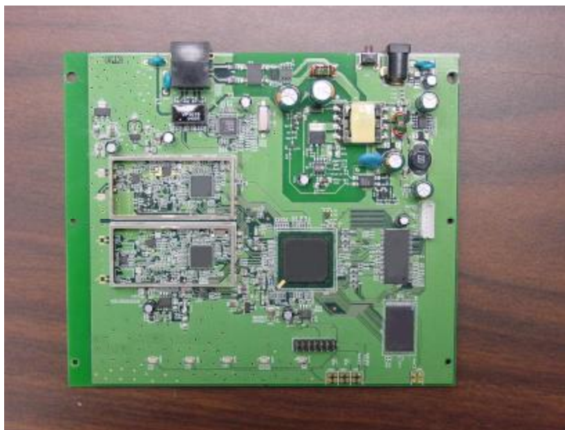
Photo 4: PCB1 top without shield
