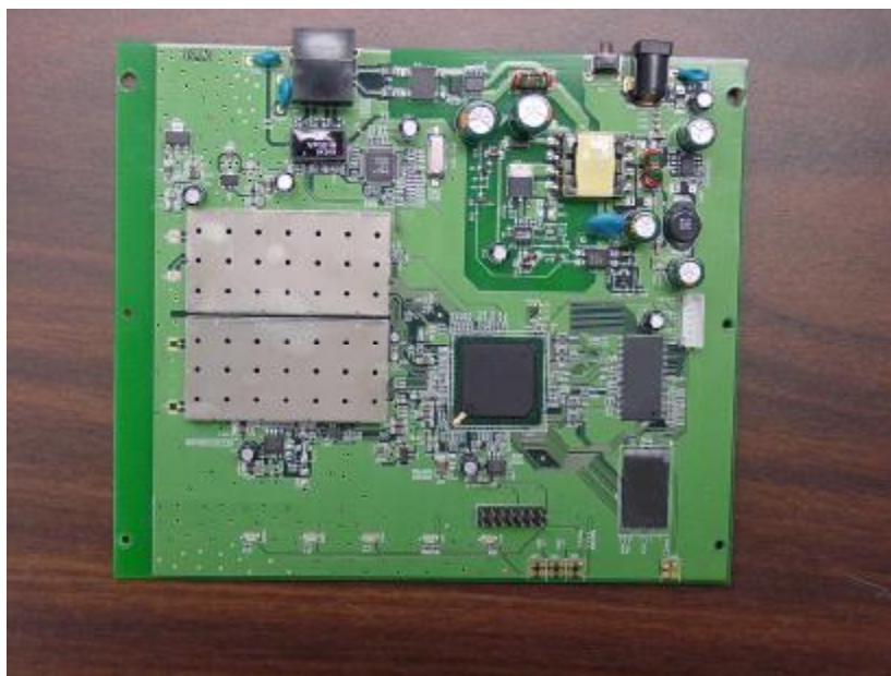
Photo 3: PCB1 top with shield
