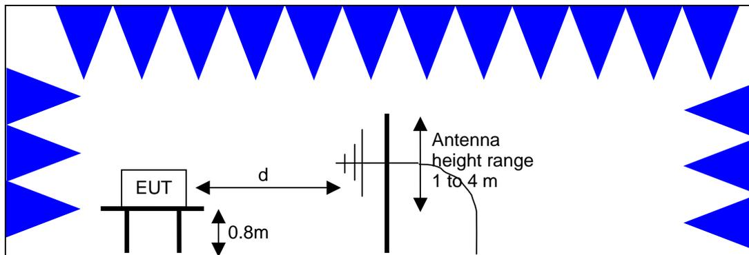
Test Configuration for Radiated Field Strength Measurements
