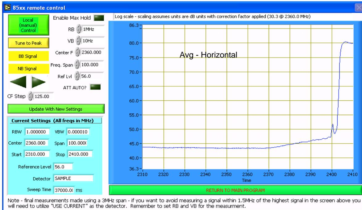
Note - final measurements made using a 3MHz span - if you want to avoid measuring a signal within 1.5MHz of the highest signal in the screen above you will need to utilize "USE CURRENT" as the detector. Remember to set RB and VB for the measurement.
