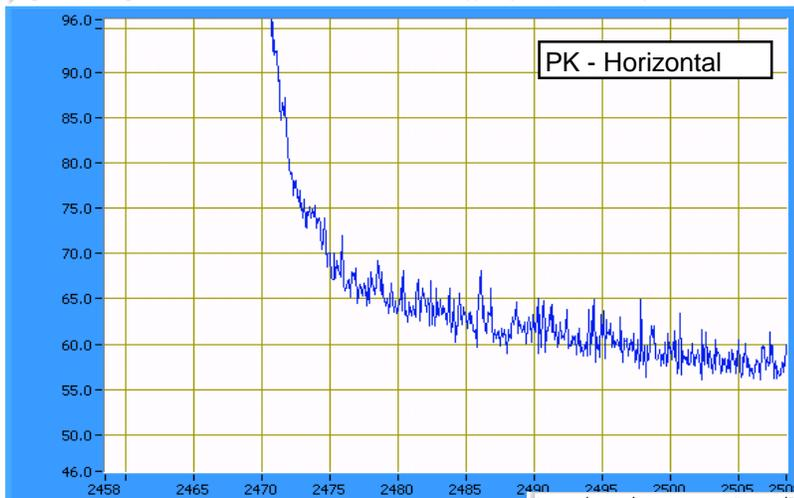
Log scale - scaling assumes units are dB units with correction factor applied (30.6 @ 2483.5 MHz)
