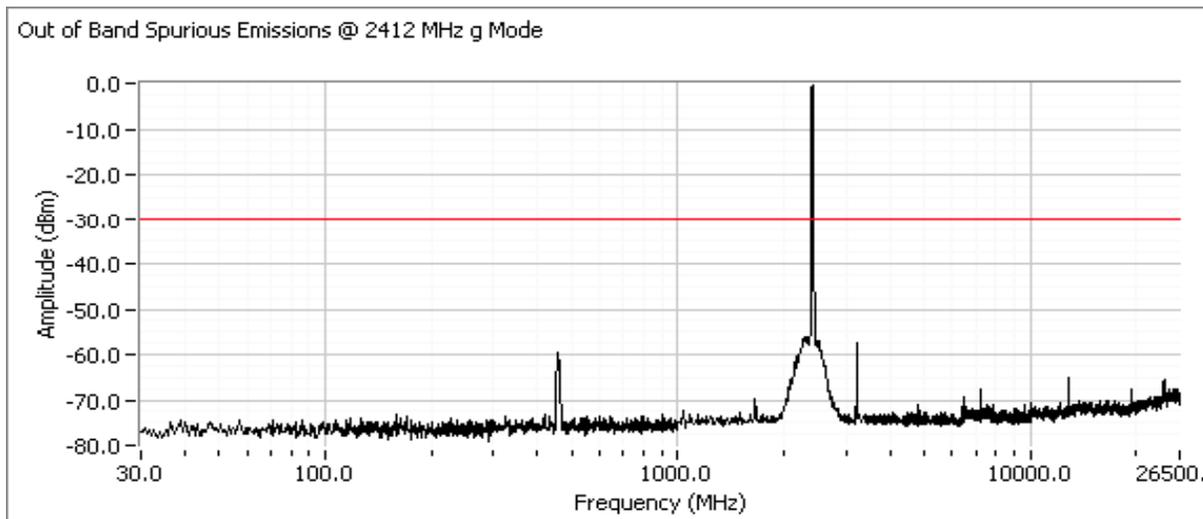
Additional plot showing compliance with -30dBc limit from 2390 MHz to 2400 MHz. Radiated measurements used to show compliance with the limits in the restricted band below 2390 MHz.
