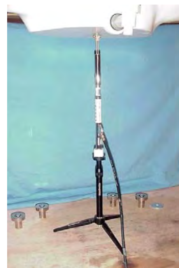
5 GHz Validation Dipole Setup
