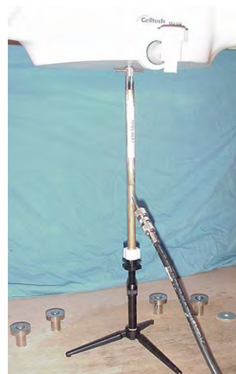
2.45 GHz Validation Dipole Setup
