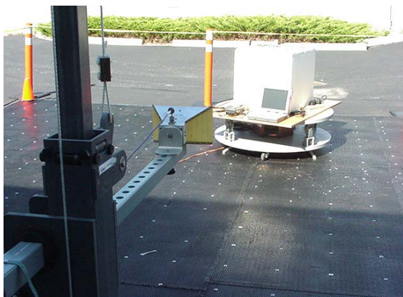
Photograph C.7-3 - Horn Receive Antenna with DUT Vehicle-Mount Antenna Configuration
