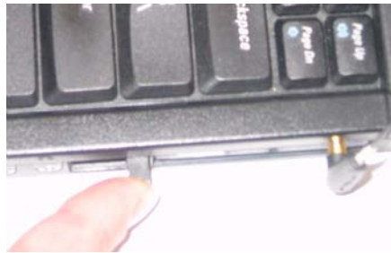
Figure 5-2: Ejecting the AirCard from its slot
