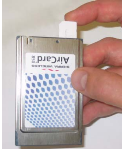
Figure 2-1: Inserting the SIM card into the AirCard SIM card slot
