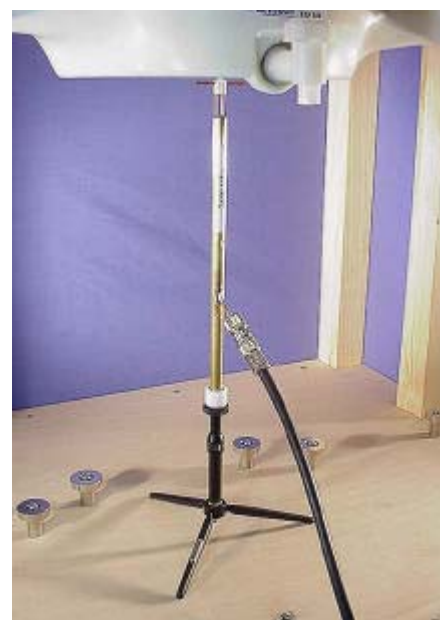
2450MHz System Check Setup Photograph
