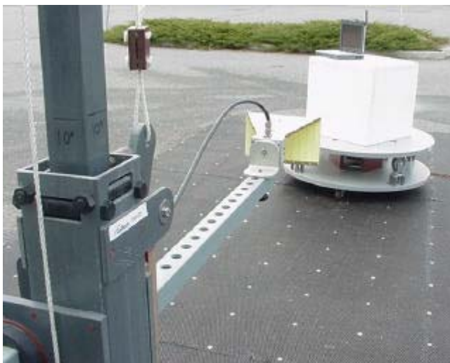
Radiated Measurement Test Setup Photograph
