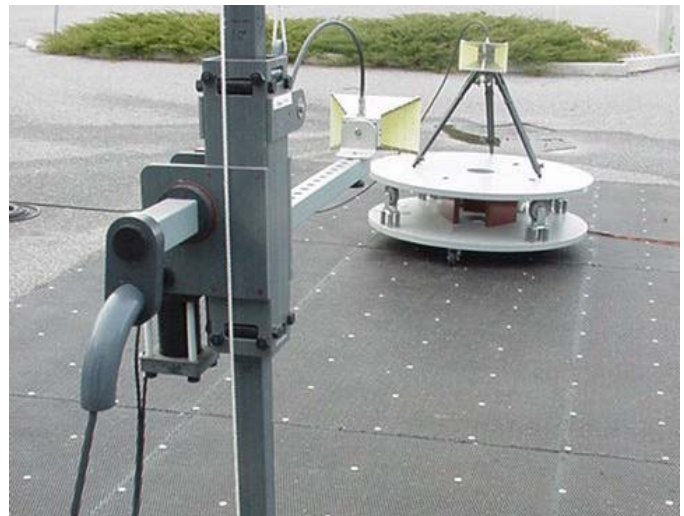
Signal Substitution Test Setup Photograph
